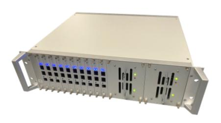
The OptiLogix HyperArray is a Very High Density Voice Packetizer for building large scale Analog, Digital Extension and E1/T1 PRI based TDM Call Recording systems.
